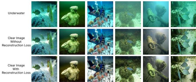
Fig. 8. **Reconstruction training objective improves restoration clarity.** Our single-step fine-tuning approach enables direct end-to-end supervision on images, aligning predicted clear and medium outputs with the dense scene-medium decomposition in Eq. (2). Real-world evaluation on [3] shows that this reconstruction loss leads to clearer restorations (bottom row), compared to outputs of the model that does not use reconstruction loss (middle row).
